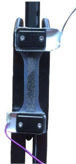
Figure 1 Stretchable Sensor attached to the Stretcher Machine
