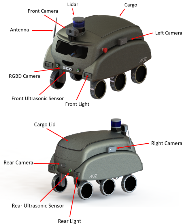
Fig. 1. An overview of BeetleBot, a multi-purpose AI-driven mobile robot and its external sensor system.
