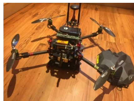
Fig. 2. The research custom build UAV Quadrotor
