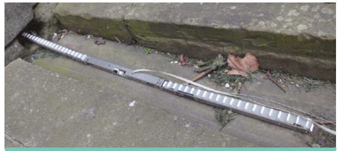
Image 3 A reconfigurable robot inspecting drains
