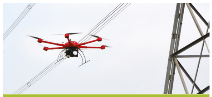
Image 2 A drone inspecting power lines
