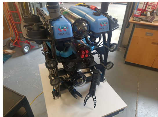
Fig. 3. AUV used for demonstration of system, a BlueRov2 heavy with an additional skid for the SLAM system and another for the 360 camera plus reach alpha manipulator.
