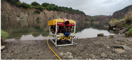
Fig. 2. An ROV equipped with AUIP mounted below.
