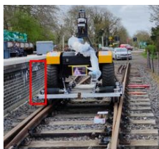
Fig. 3. Congested space between the track and platform on the right side
