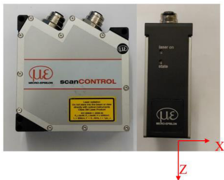
Figure 4. Image showing the laser scanner co-ordinate system.
