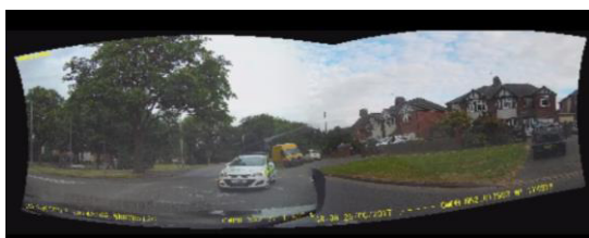
Figure 5. Image stitching distortion
