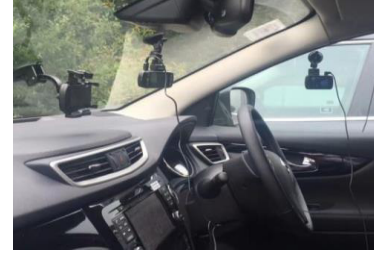
Figure 3. Camera settings from inside the autonomous vehicle
