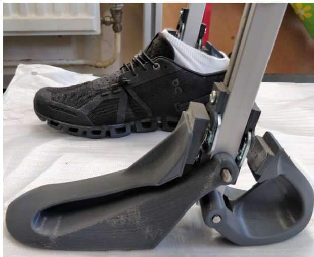
Figure 15: Ankle joints of SARAH with and without shoe.
