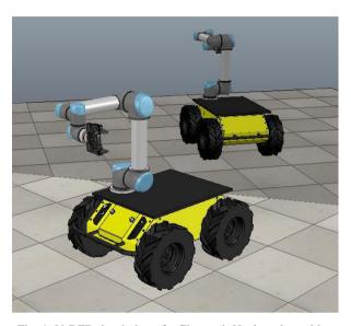
Fig. 1. V-REP simulation of a Clearpath Husky robot with a UR5 robot arm mounted to it.
