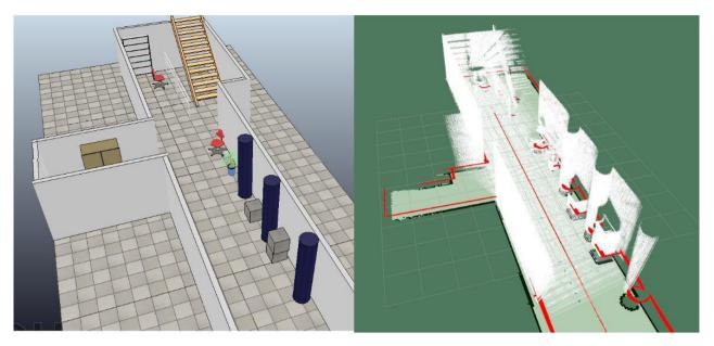
Fig. 4. (left) initial test scene created in VREP (right) Simulated 2D Lidar and depth sensor data combined in Rviz. Created by the mobile platform moving in a straight line in a single direction in simulation.
