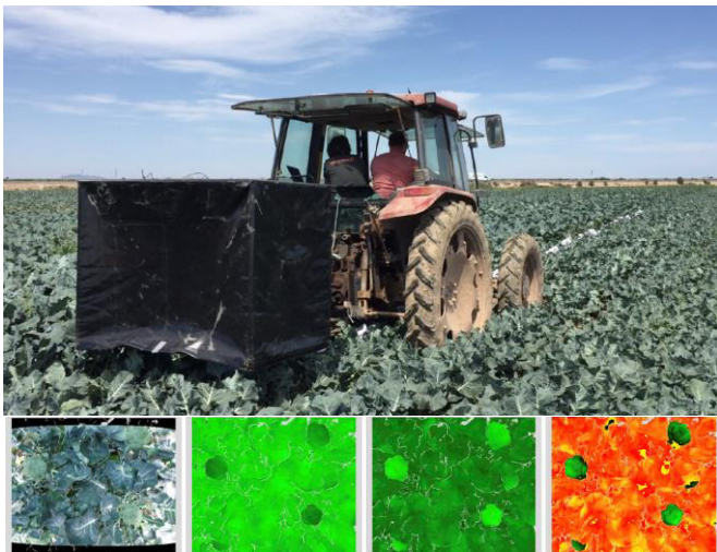
Figure 1. Top: Data acquisition with the 3D sensor mounted at the rear of the tractor. The sensor is fixed inside a purpose-built “black box” enclosure to block direct sunlight and other external incidences. Bottom: 3D point cloud images of broccoli plants (far left) are analyzed offline based on local angular features (middle frames) to segment broccoli heads (far right).
