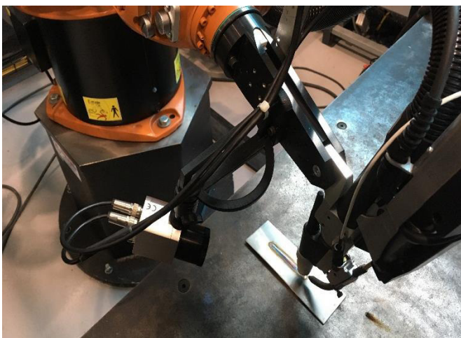
Figure 1. The welding components on the end effector of the robotic arm
