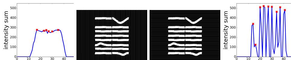
Fig. 1: Perpendicular lines drawn on the binary image at angle 0^\circ (left) and 90^\circ (right), along with their oriented graphs of intensity sums.
